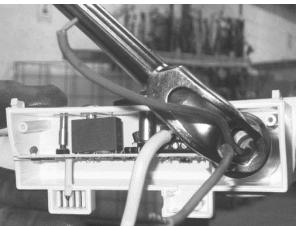
Put the unit in place, with its nut, then tighten it up.
