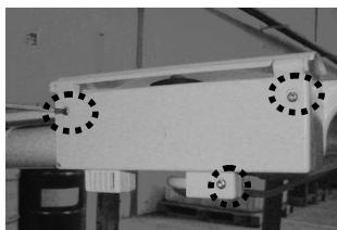
Unscrew the three screws with the torx screwdriver.
