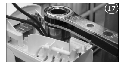
Finish tightening the nut to 25 N.m with the torque wrench.
