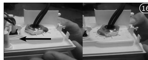
Push the whole unit up to the top of the appliance, until it reaches the end-stop on the body.
