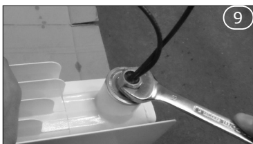
Loosen the heating element with the flat 18mm spanner (take care to keep the appliance steady, to prevent any oil spillage). Finish unscrewing the heating element manually.
