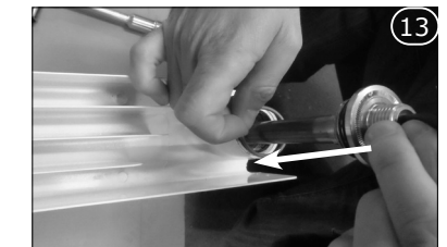
Insert the heating element into its compartment. Tighten the heating element to 50 N.m with the torque wrench.
