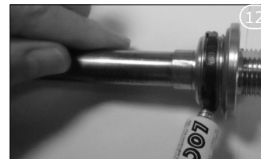
Put the sealing paste onto the new heating element.
