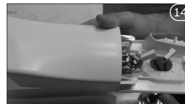
Replace the unit onto the body of the appliance, taking care to make sure the connectors go properly into the hole provided. Lower the unit until it reaches the end-stop on the heating element.
