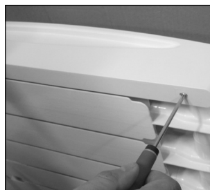
Unscrew the screw on the right side facing you.
