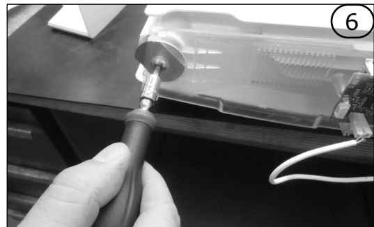
Unscrew from the opposite side of the element with the hexagonal spanner.
