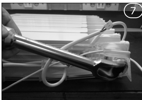
Release the nut on the left with the 27mm spanner.
