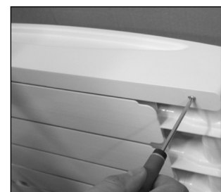
Screw up the end panel. The appliance is ready to put in place.
