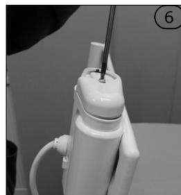
Screw up the lower part of the casing of the cylindrical receiver using the torx screwdriver T10.
