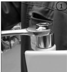
Release the heating element with the 24mm spanner (take care to keep the appliance steady, to prevent any oil spillage). Finish unscrewing the heating element manually.
