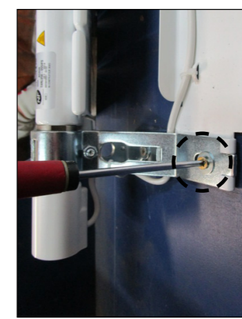
Completely unscrew the 4 "exposed" screws (two screws at the top on the plate and another screw inside the appliance for the upper and lower rotary units).
